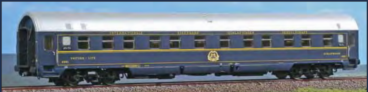
Carrozza letti UHansa con mantici e carenatura originale della CIWL immatricolata presso il Parco FS. Sleeping car UHansa, owned by CIWL, with original ends and side skirt, registered in Italy. Typ UHansa Schlafwagen, Originallackierung bei der FS eingestellt.
