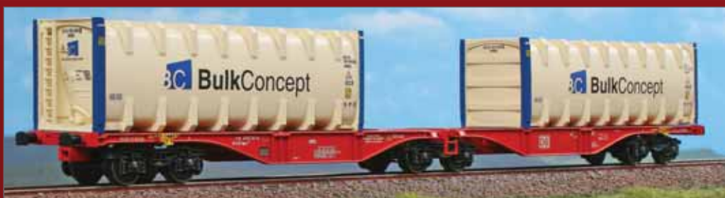
Carro intermodale articolato Tipo Sggrss 80' DB con carico di bulk. Articulated container wagon Type Sggrss 80' of DB with bulk. Gelenk-Containertragwagen Typ Sggrss 80' der DB mit Bulk.
